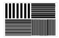
Each of the sets of parallel lines is precisely machined onto a plastic sheet. The lines are filled (cast) with Cerrobend® high-density metal alloy. This causes the gamma radiation to be attenuated, thereby providing the QA image.
