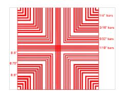
Each of the sets of parallel lines is precisely machined onto a plastic sheet. The lines are filled (cast) with Cerrobend® high-density metal alloy. This causes the gamma radiation to be attenuated, thereby providing the QA image.
