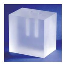
During standard clinical conditions, the deadtime is a function of the scatter within the radiation source and its immediate surroundings. The phantom provides the simulated characteristics of forward and back scatter of the <sup>99m</sup>Tc gamma rays and allow the measurement\* of the camera's deadtime.
