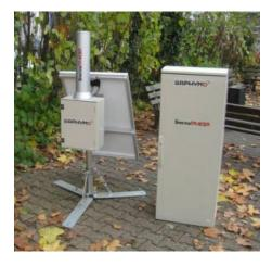
The SpectroTRACER produces a spectroscopic analysis of the detected nuclides identification. The SpectroTRACER is used for the measurement of radioactivity when a standard gamma dose rate monitor is not efficient enough and when it is necessary to discover the nature of the gamma radiation.
