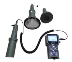
Together with the probes, SaphyRAD MS allows to cover most of the needs of first responders. SaphyRAD MS associates a wide range dose rate meter and external smart probes for source and hot spot search and contamination measurement.
