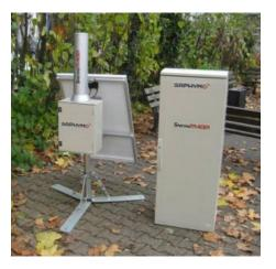
The SpectroTRACER produces a spectroscopic analysis of the detected nuclides identification. The SpectroTRACER is used for the measurement of radioactivity when a standard gamma dose rate monitor is not efficient enough and when it is necessary to discover the nature of the gamma radiation.
