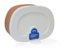
Abdominal imaging is useful for diagnosing disease and monitoring treatments. The Model 057A is representative of a small adult abdomen and can be imaged under CT, MR and ultrasound. This feature makes the phantom a useful tool for applications such as image fusion studies; imaging protocol developments; scan technique training; and system testing, validation and demonstration.
