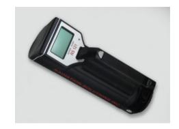
GeoView provides specificated views on accumulated data such as survey in both doserate or cps. The RT-22 Handheld Radiation Detector can be connected with the software through USB or Bluetooth.
