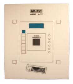
The CR/DR Test Tool incorporates a variety of testing parameters that, when used daily, tracks geometry (region of interest) symmetry, line pair resolution, as well as low and high contrast performance. Measurements of the various targets allow for evaluation of both the monitor and printed film image. The CR/DR tool will become a valuable asset to the QA technologist and the medical physicist trying to determine the source of an image quality problem or complaint.
