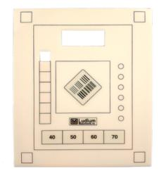
The L-777-Mini is used to make a sample image of the approved system. This image is saved and used as a benchmark for future evaluation of the system. Frequency of the future evaluations of the image system are determined by the QA manager. Testing can be performed daily, weekly, or as directed by the medical physicist or quality assurance manager. The more frequent the testing the less likely a negative trend will develop.
