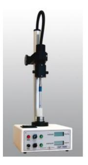
The Single Mast Electrodeposition Equipment – EDP 7000 system is the most efficient principle for trapping a radio-element in liquid solution. This principle allow to deposit the radio-isotopes contained in a solution onto a metallic plate. To measure the quantity of radio-element trapped, the metallic plate is afterwards placed into a suitable machine (spectrometer or other one).
