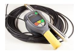
The instrument is specifically calibrated to measure an accurate direct reading of the percentage of potassium-40 in the surrounding environment. The detector probe is particularly suitable for placement in boreholes.
