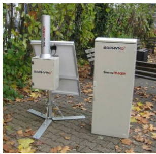
ShortLINK Short- Range Environmental Radiation Monitoring Network - Bertin/ Saphymo
