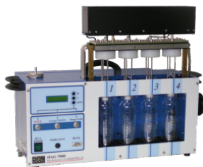
Carbon 14 Sampler with 4 Vials - SDEC
