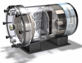
Model 610 AAPM CT Performance Phantom - CIRS
