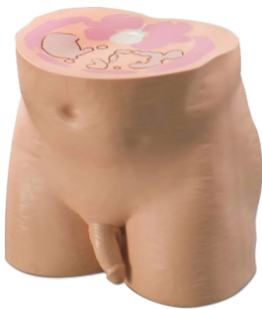
Model 038 STEEV Steriotactic End-to-end Verification Phantom Patient
