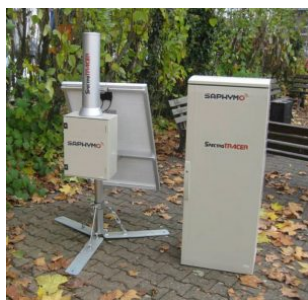
GammaTRACER Spider Autonomous Gamma Monitor for Emergencies - Saphymo
