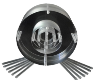
Model 468 - CT Dose Index Phantom - Sun Nuclear
